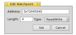
As can be seen here, the watchpoint can be triggered either via a read or a write, and one can specify how many bytes away from the current address can be written to while still triggering the halt.
